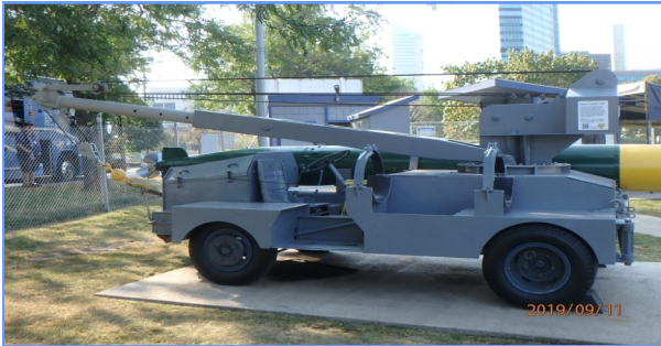
Mark 14 Steam driven Torpedo
