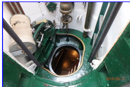
Escape Trunk Hatch
